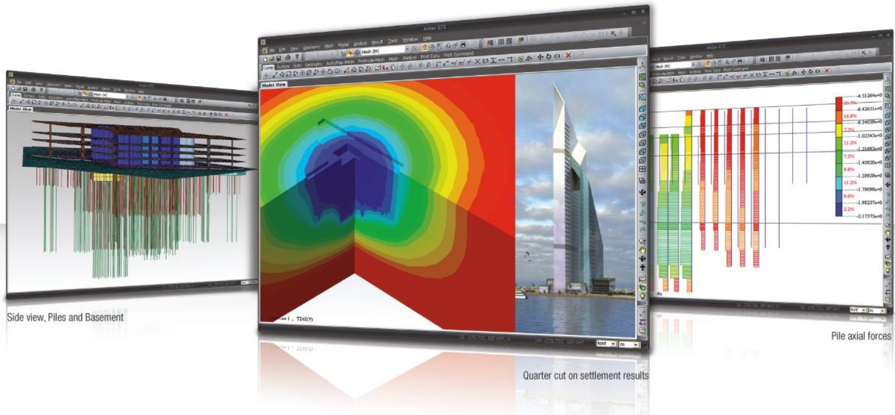
Located in Doha, Qatar, Dubai Tower piled raft analysis
